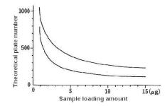
$\label{eq:column} \begin{array}{l} \mbox{Column : ULTRON ES-OVM ( 4.6mm $\phi$\times$150mm )} \\ \mbox{Mobile phase : 20mM KH_2PO_4 (pH=5.5)/C_2H_5OH= 100/4} \\ \mbox{Flow rate : 1.0 mL/min.} \\ \mbox{Column temp. : 25 $^{\circ}$C} \\ \mbox{Detector : UV-254nm} \\ \mbox{Injection Volume : 0.5 $\mu$L} \\ \mbox{Sample : Tolperison} \end{array}$
